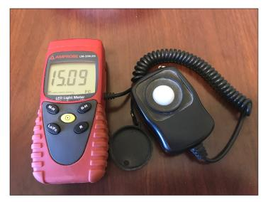
Figure 1. LED light meter used to measure light level.
