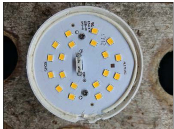
Figure 2. LED lamp with globe removed to show LED chips.
