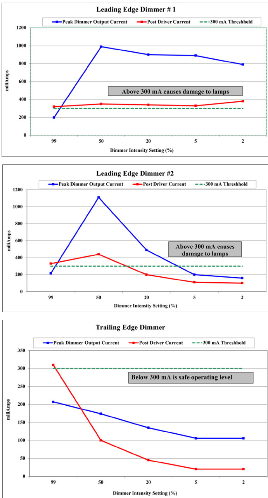
Figure 3. Current outputs of leading-edge and trailing-edge poultry house light dimmers.
